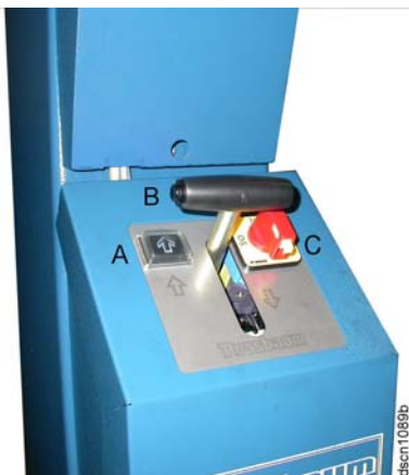
Pic 1: A button "lifting" B lever "lowering" + button "unlocking the ratchets" C main switch
